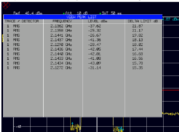
Fig. 4-35 Measurement of the peak list for the spectrum emission mask
