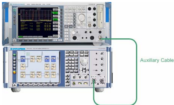
Fig. 3-3 Test setup during normalization
